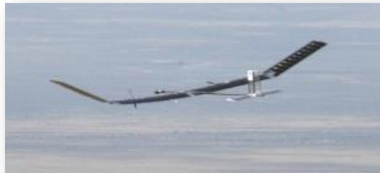
Zephyr flight - 11/07/2018 Solar drone, 70000ft alt. >25 days continuous flight World record at Maiden flight
